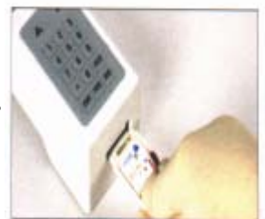
Insert cartridge into hand-held analyzer.
